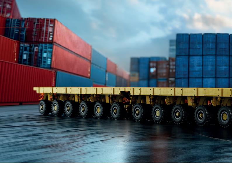
SEAL SPMT is engineered to meet the heavy-duty transportation needs of large-scale components such as ship structures, construction equipment, bridges, and wind turbines. It is equipped with a load balancing system, high maneuverability, a modular design, and a self-propelled drive system.
